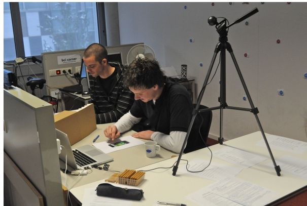
Figure 7.4: Test set-up showing positions of participant, paper prototype and controller, laptop screen and over-the-shoulder camera
